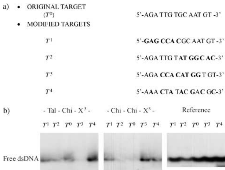
Fig. 5. a) Modified targets used in specificity assays (as double strands, in combination with the respective complementary sequence). b) Specificity tests: Gel-retardation experiments with the original target ( T^0 ) and four modified targets ( T^1 , T^2 , T^3 , and T^4 ). The general structure of the peptides is Ac-Arg-Ual-Sar-Chi-X 2 -X 3 -Arg-NH 2 and Ac-Arg-Ual-Sar-Tal-X 2 -X 3 -Arg-NH 2 . In the reference lanes, no peptide mixture was added. The total concentration of the mixture of twelve peptides was 1 mM in each case.
